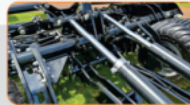
Machine tilt system with two reinforced cylinders
